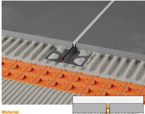
Schlüter-DILEX-FCS is a narrow, prefabricated movement carrier profile with lateral, trapezoid perforated anchoring legs and is made of recycled rigid PVC. The lower movement zone and the orange protective covering consist of soft CPE.
