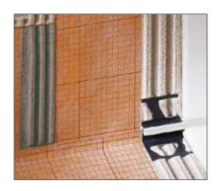
Schlüter-KERDI is a crack bridging waterproofing membrane made of soft polyethylene, with a special fleece fabric on both sides for effective anchoring in the tile adhesive. Schlüter-KERDI was developed as a waterproofing membrane for bonded assemblies with floor and wall coverings made of tiles and natural stone.
