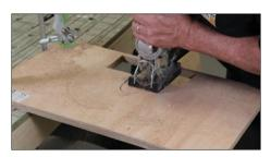
Following the outline of the drawn shape, cut the opening into the piece of plywood.
