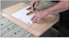
O Position the piece of sub-floor created in steps A & B over a further piece of 18mm exterior grade plywood, approximately 500mm long, lining up the ends of the plywood pieces that will be fitted nearest to the wall. Doing this will create a 'ledge' for the part of the sub-floor referred to in steps 16 & 21 to sit on and be secured to. Use the cut-out in the top piece of plywood to draw the shape onto the bottom piece of plywood.
