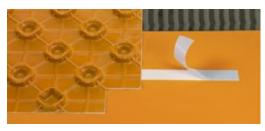
The levelling panel Schluter-BEKOTEC-EN12FGK must be used in doorways. It must be fitted underneath the adjacent studded panel(s) and bonded to the substrate with a C2 or C2F classification cementitious tile adhesive using a 6 x 6 mm notched trowel. It is adhered to the underside of the studded panel(s) using the BTZDK66 double-sided tape.
