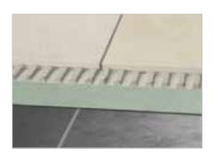
Schlüter-REFLEECE is a fleece mat made of recycled PET with a bonding layer laminated on the underside. It is suitable for creating easily removable floor coverings made of tiles and natural stone. The self-adhesive underside easily detaches from the substrate during removal without damaging the sub-floor. (Product data sheet 20.1)
