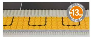
Schlüter-DITRA-HEAT-E-DUO further optimises the proven electrical floor heating system. The integration of a reinforced, 2 mm fleece fabric on the underside of the membrane drastically reduces heat radiation into the substrate. The thermal barrier on the membrane's underside enables a significantly faster heat-up response in the covering without any change in the low energy supply and offers certified impact sound reduction of up to 13dB.
