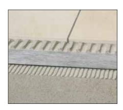
**Schlüter®-DITRA-SOUND** is a 3.5 mm thick bonded impact sound insulation product made of heavy polyethylene mat for tile coverings. A fleece fabric is laminated on both sides for bonding with the tile adhesive.
