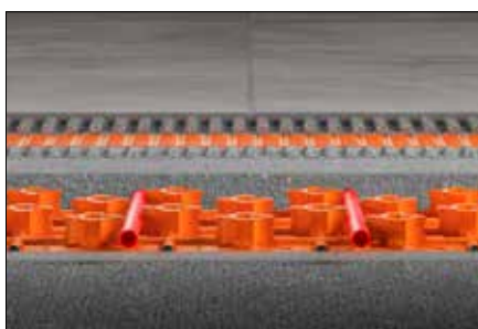
Schlüter®-BEKOTEC-EN 18 FTS with pre-adhered sound insulation
