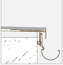
The assembly shown here only applies to cantilevered balconies and ground level terraces (with modified edge assemblies).
