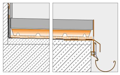
The assembly shown here only applies to cantilevered balconies and ground level terraces (with modified edge assemblies). Roof terrace assemblies must comply with all technical standards for insulation and waterproofing as specified in DIN 18531.
