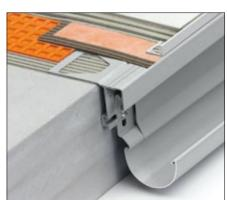
Schlüter®-BARIN as a drainage channel in a balcony construction with Schlüter®-DITRA-DRAIN as a drainage assembly and the Schlüter®-BARA-RTKE balcony finishing profile.
