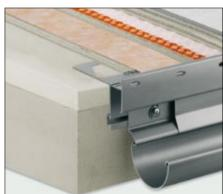
Schlüter®-BARIN gutter in a balcony assembly with a bituminous waterproof membrane. The Schlüter®-TROBA-PLUS drainage membrane and screed are placed above the waterproofing layer. The tiles are installed in the thin-bed method over the Schlüter®-DITRA uncoupling and waterproofing membrane.
