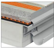
Schlüter®-BARIN acting as a drainage channel for a balcony assembly with bitumen waterproofing. The area drainage system Schlüter®-TROBA and a load distribution layer of gravel or crushed stone are laid on top. Large format pavers are loosely installed over it.
