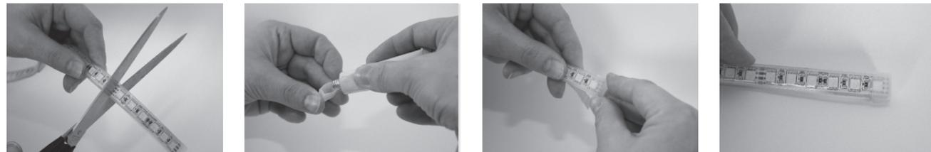
1. Cut the IP-protected LED strip at the marked points.
