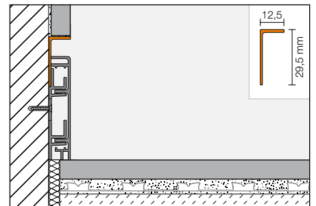
Shadow joint angle profile Schlüter®-DESIGNBASE-CQ/SG
