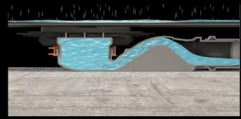
High flow rate causes self-cleaning effect
